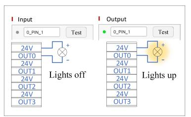
Figure 3- 17 Output signal application diagram
