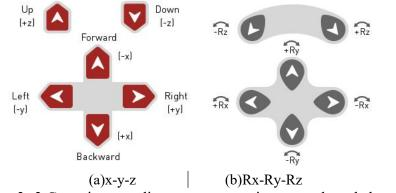
Figure 3- 3 Cartesian coordinate system motion control mode button
