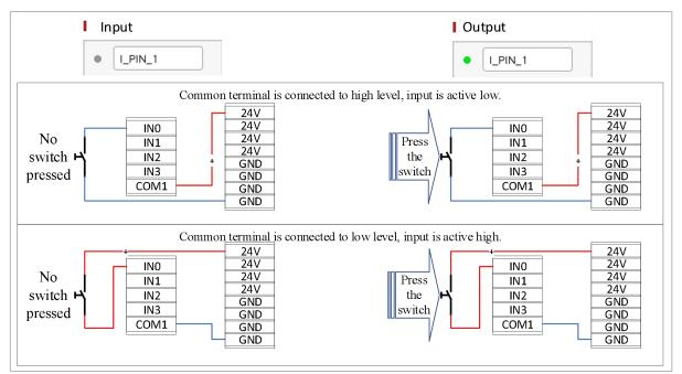
Figure 3-16 Input signal application diagram
