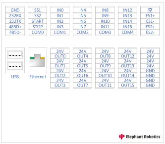
Figure 3-15 Input and output interface description
