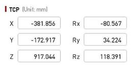
Figure 3-10 Coordinate position display window
