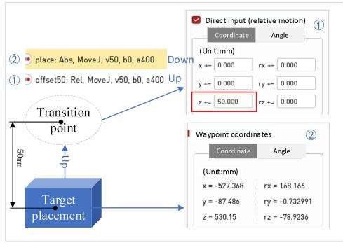
Figure 4- 6 Application examples of direct input coordinate values
