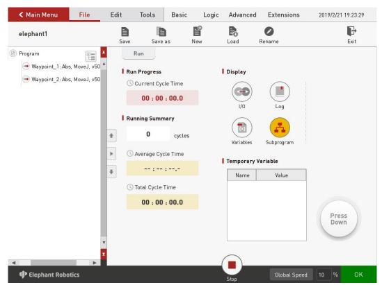
Figure 5-15 Manual mode to debug the program
