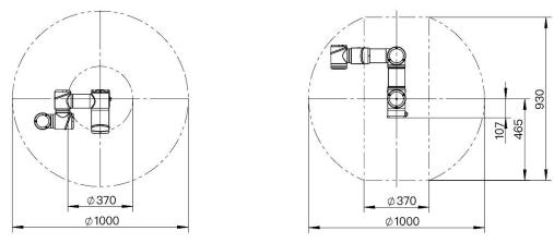
Figure 2- 3 Schematic diagram of the Panda 3 workspace
