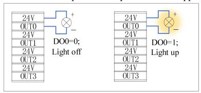
Figure 3- 10 Output application example diagram
