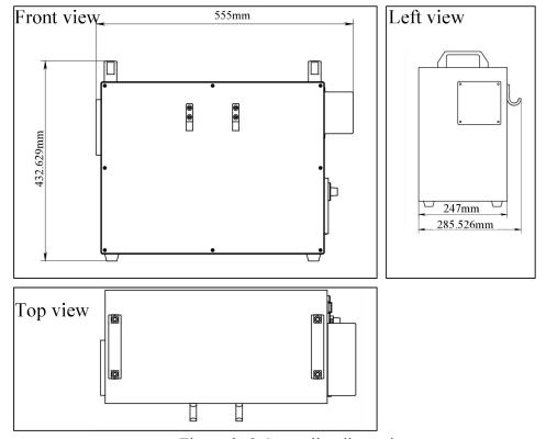
Figure 3-2 Controller dimensions
