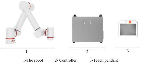
Figure 2- 1 Robot system
