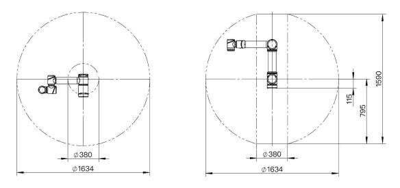
Figure 2- 4 Schematic diagram of the Panda 5 workspace
