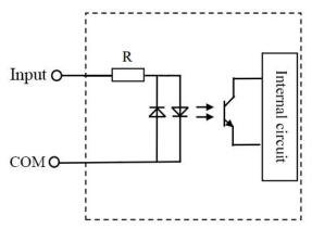
Figure 3-7 Digital input port schematic
