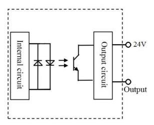
Figure 3- 9 Digital output port schematic
