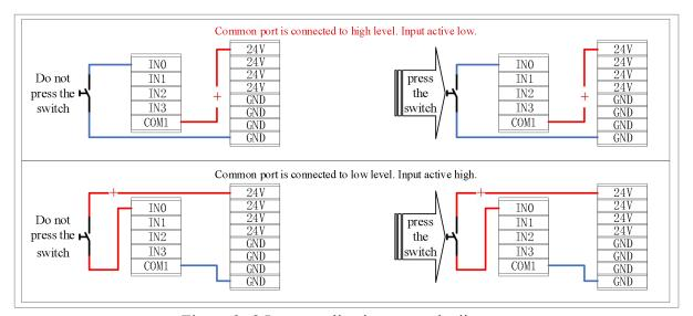
Figure 3-8 Input application example diagram
