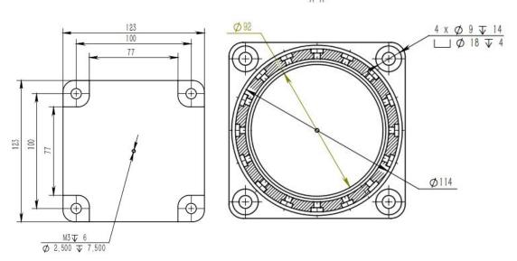
Figure 3-1 The specific hole size
