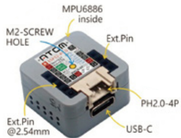
Atom pin diagram
